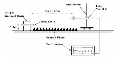
The radiated emission tests were performed in the 3 meters chamber test site, using the setup accordance with the ANSI C63.10-2013. The specification used was the FCC 15.209, FCC 15.407 and RSS-247, RSS-Gen limits.
