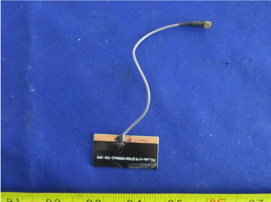
EUT- ADS-B Antenna View
