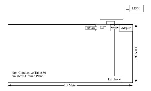
Battery Power supply(Radiation Test):
