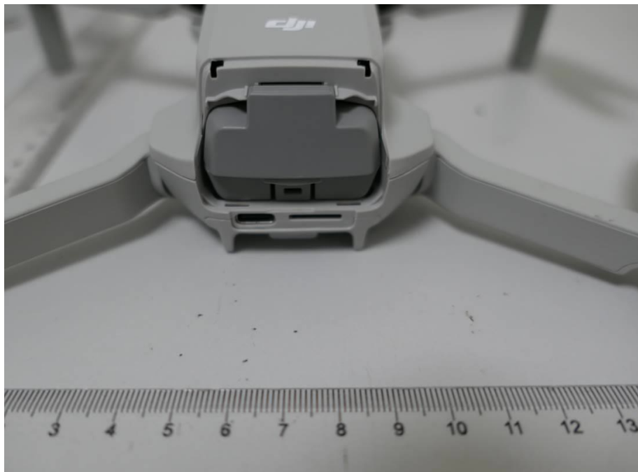
Figure 4: External view 4 – rear with battery cover removed
