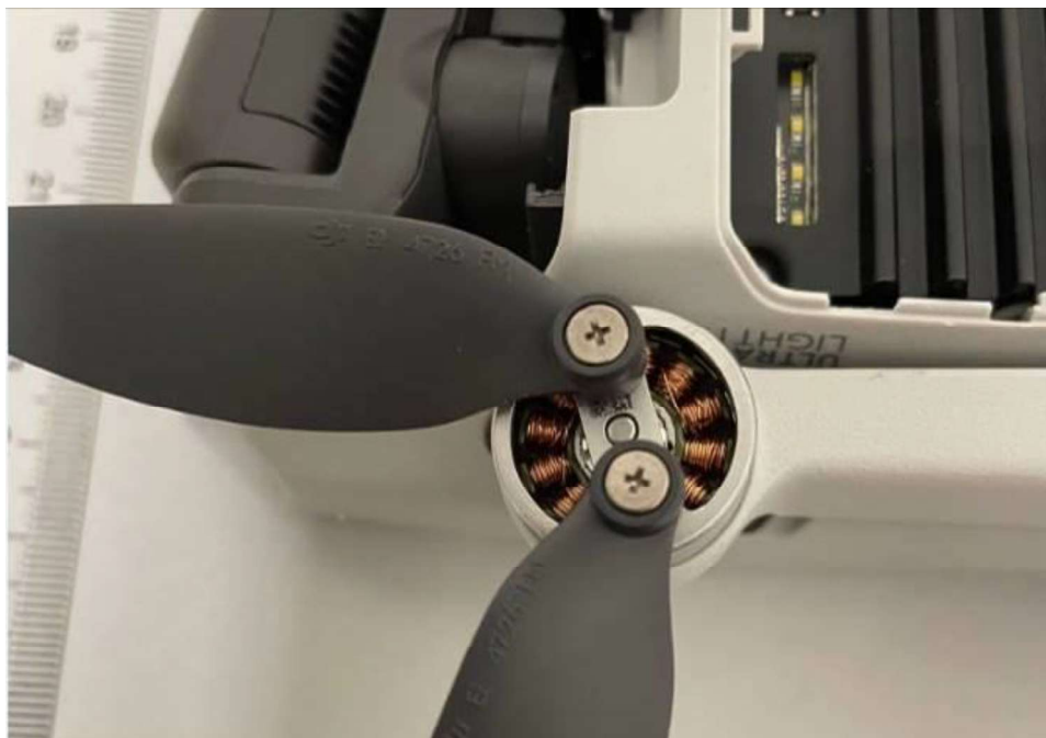
Figure 18: Internal view (Propeller motor view)
