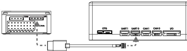
When using the M210/M210 RTK flight platforms, connect the OSDK port on the left of the expansion ports on the aircraft to the UART port on the Manifold 2. Make sure to use the UART Cable for M210 Series included.
