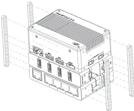
2. When using with DJI flight platforms, mount the Manifold 2 and other external devices to the flight platform using a compatible mounting bracket.
