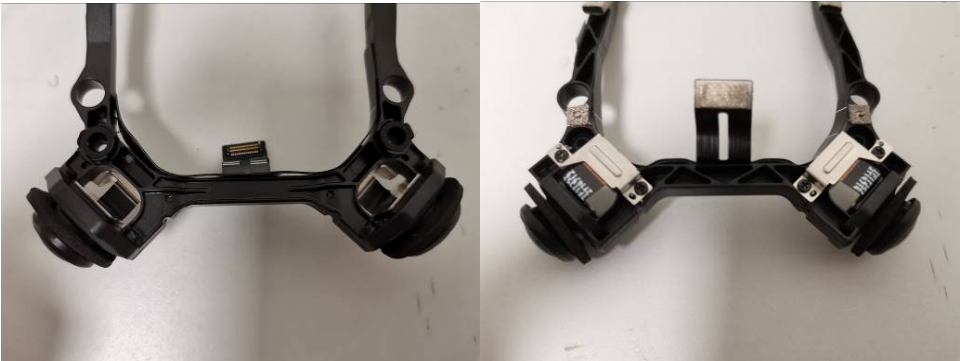
Figure 5: Internal view for front vision system
