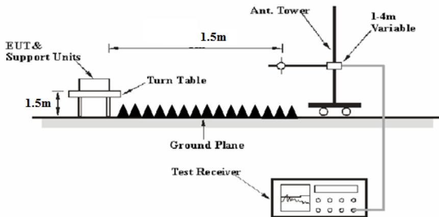
The radiated emission below 1GHz tests were performed in the 3 meters chamber test site A, above 1GHz tests were performed in the 3 meters chamber test site B, using the setup accordance with the ANSI C63.10-2013. The specification used was the FCC 15.209, and FCC 15.407 and RSS-247, RSS-Gen limits.
