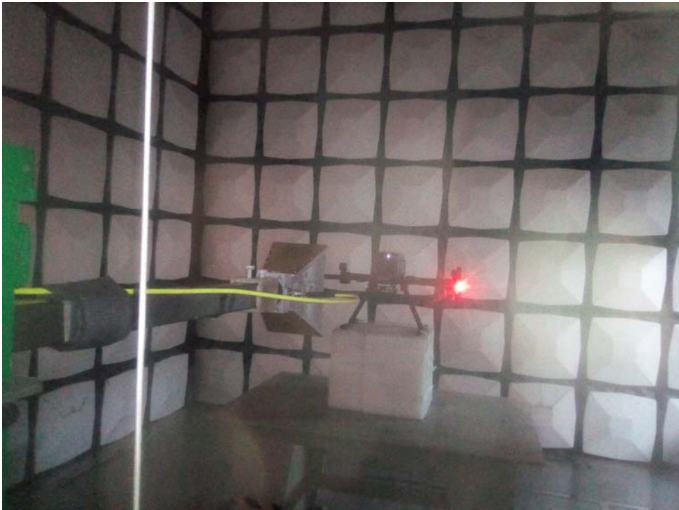
Radiated Emission Above 1GHz View
