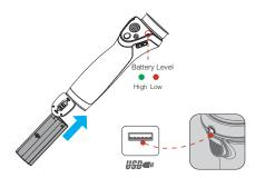
To charge the Osmo Mobile, connect the USB adapter (not included) to the charging port using the provided power cable.
