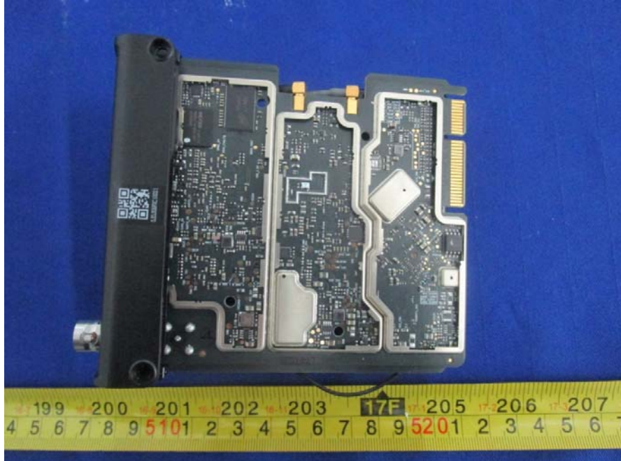
EUT – RF Board Bottom Unshielded View
