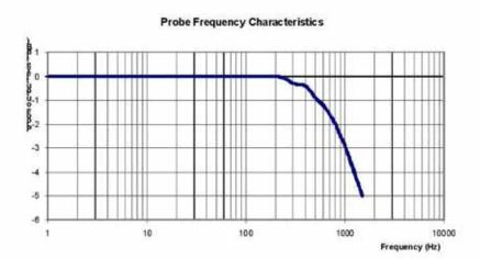
Video Bandwidth at 500 Hz 1 dB Video Bandwidth at 1.02 KHz: 3 dB
