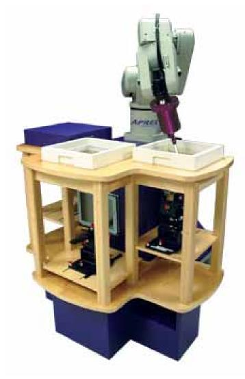
Where the system identifies multiple SAR peaks (which are within 25% of peak value) the system will provide the user with the option of assessing each peak location individually for zoom scan averaging.
