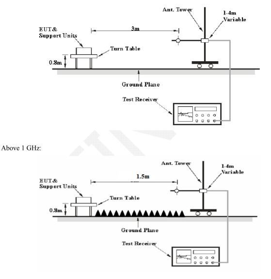
The radiated emission and out of band emission tests use the setup accordance with the ANSI C63.4-2009. The specification used was the FCC 15.209/15.205 and FCC 15.249 limits.
