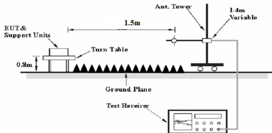
The radiated emission and out of band emission tests use the setup accordance with the ANSI C63.4-2003. The specification used was the FCC 15.209/15.205 and FCC 15.249 limits.
