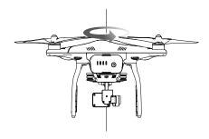
Hold the aircraft vertically, with nose pointing downward, and rotate it 360 degrees around the center axis. Recalibrate the compass if the Aircraft Status Indicator glows solid red.
