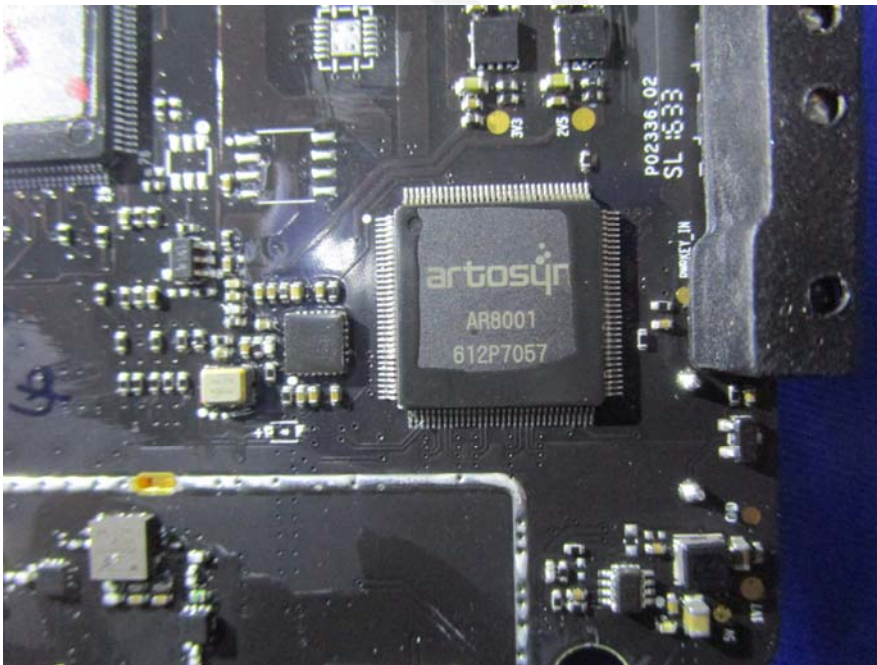
EUT – Main Chip View
