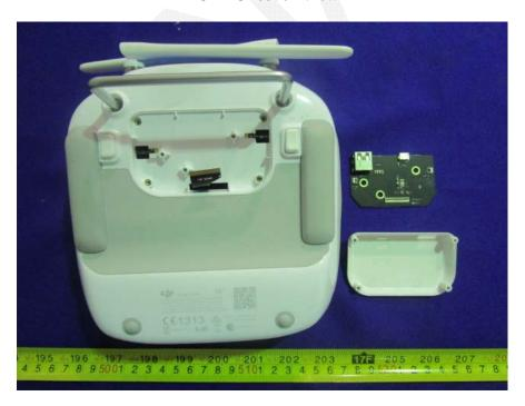
**EUT – Control Board Top View**
