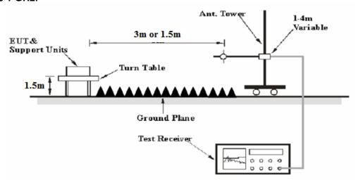
The radiated emission tests were performed in the 3 meters chamber, using the setup accordance with the ANSI C63.10-2013. The specification used was the FCC 15.209, and FCC 15.407 limits.
