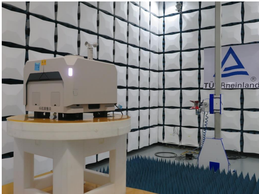
Photograph 2: Set-up photo for Radiated Emission, Above 1GHz
