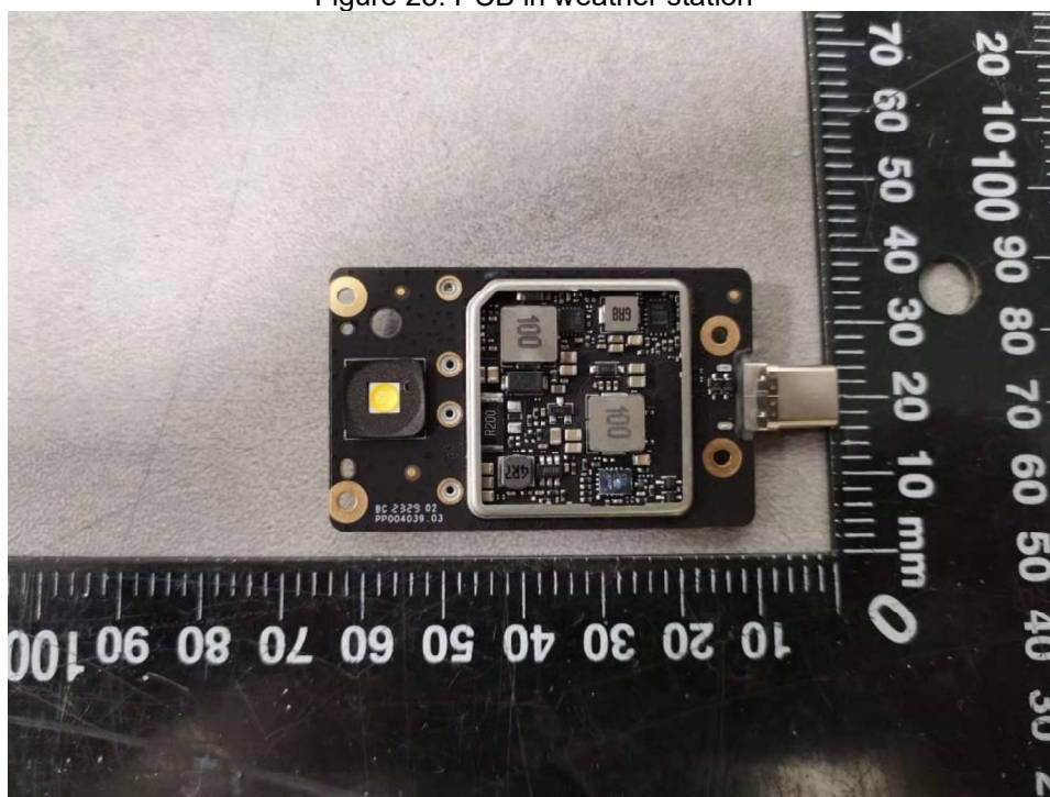
Figure 24. PCB in weather station (metal shield cover removed)
