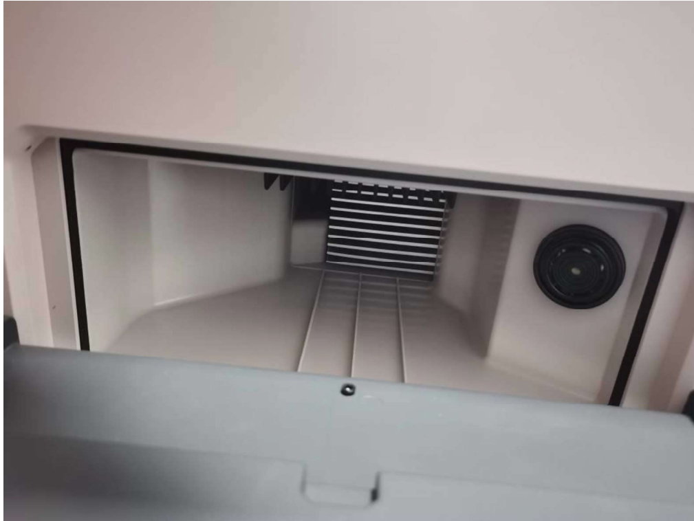
Figure 15. Heatsink in venting tunnel
