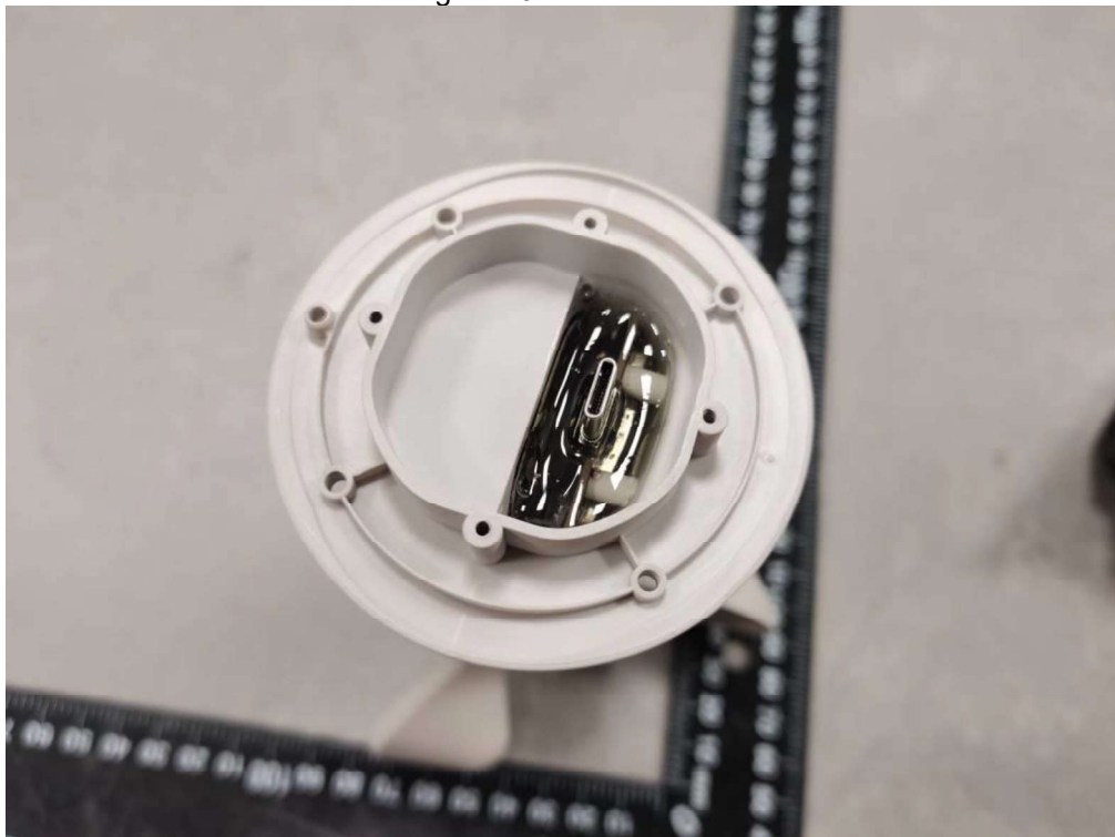
Figure 20. Weather station with potting
