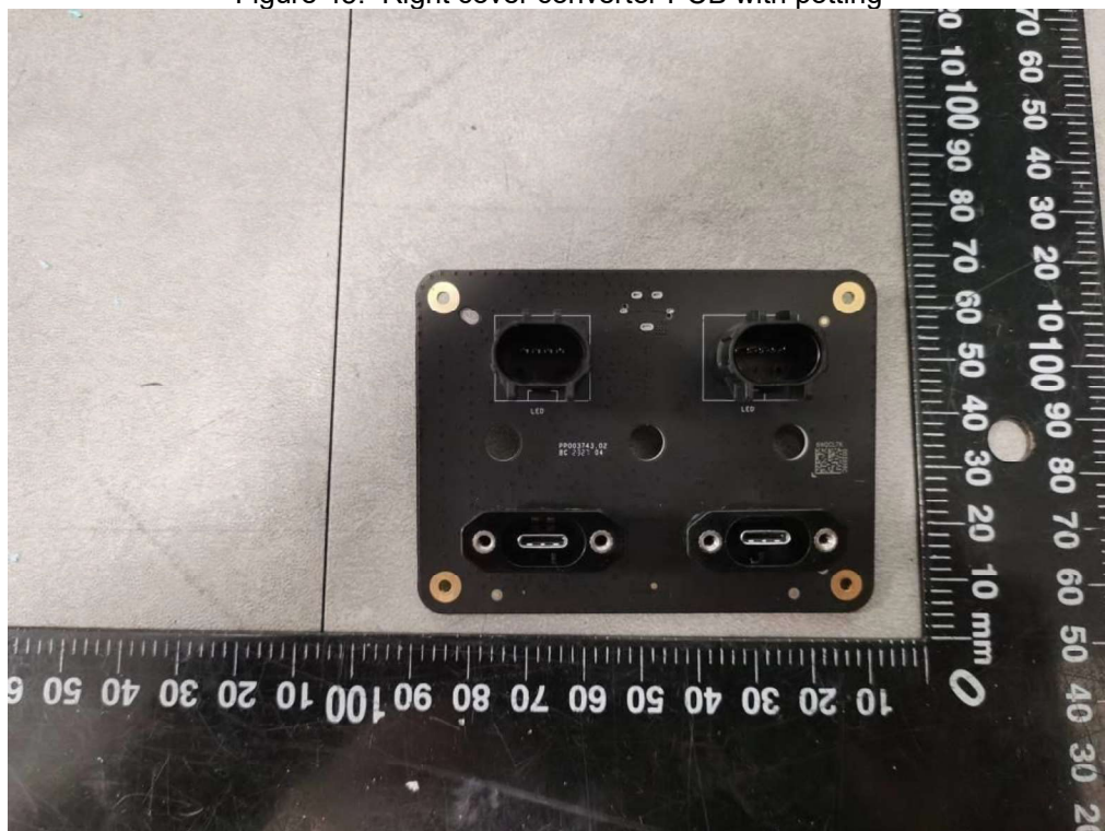
Figure 46. Right cover converter PCB with potting removed
