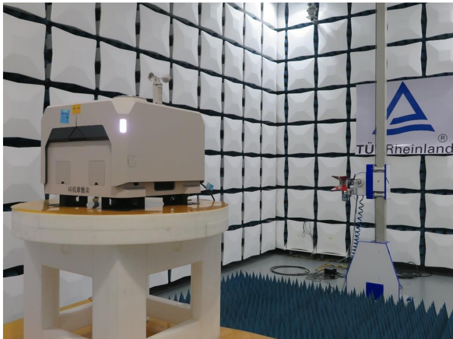
Photograph 2: Set-up photo for Radiated Emission, Above 1GHz
