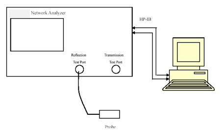
Liquid Verification Setup Block Diagram
