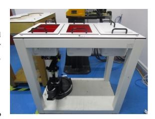
A white cover is provided to cover the phantom during off-periods to prevent water evaporation and changes in the liquid parameters. Free space scans of devices on top of this phantom cover are possible. Three reference marks are provided on the phantom counter. These reference marks are used to teach the absolute phantom position relative to the robot.
