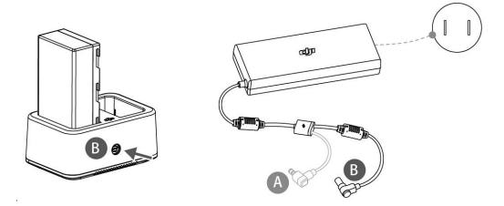
Tips: The charging hub can charge two batteries at the same time. It will take a longer time to charge the Intelligent Flight Battery and remote controller together.
