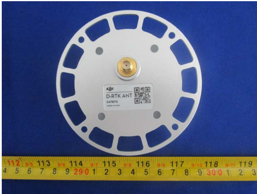
EUT- GPS Antenna Bottom View
