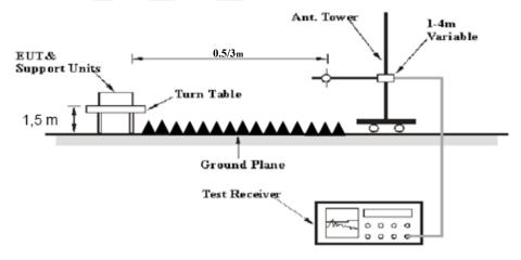
The radiated emission and out of band emission tests were performed in the 3 meters chamber test site, using the setup accordance with the ANSI C63.10-2013 The specification used was the FCC 15.209/15.205 and FCC 15.249 limits.
