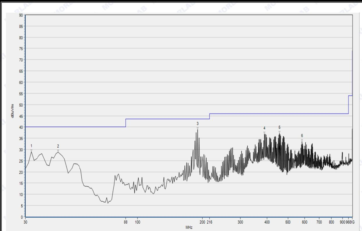
(Plot A: 30MHz – 1GHz, Test Antenna Vertical)
