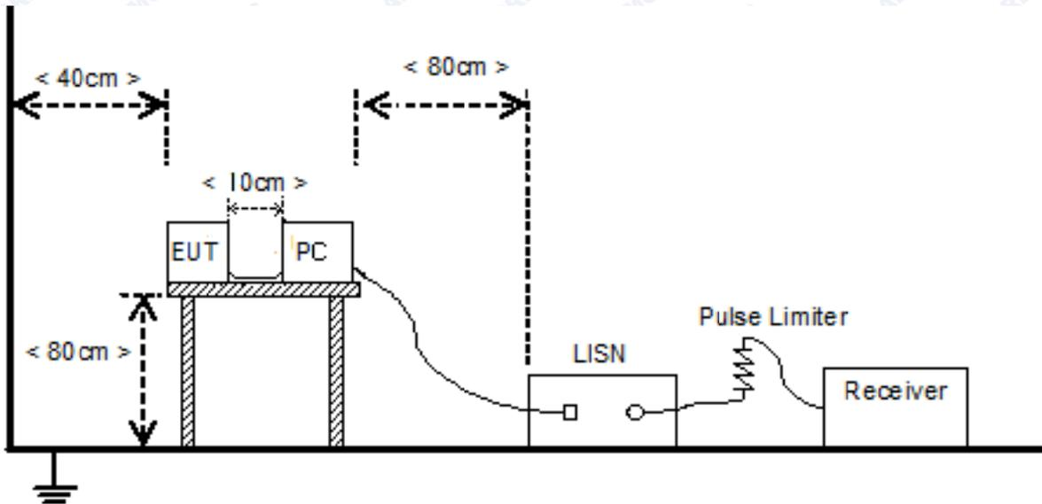
The EUT is placed on a 0.8m high insulating table, which stands on the grounded conducting floor, and keeps 0.4m away from the grounded conducting wall. The EUT is connected to the power mains through a LISN which provides  $50\Omega/50\mu\text{H}$  of coupling impedance for the measuring instrument. A Pulse Limiter is used to protect the measuring instrument. The factors of the whole test system are calibrated to correct the reading.
