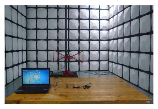
Radiated Emission View (Above 1GHz) -Battery Mode
