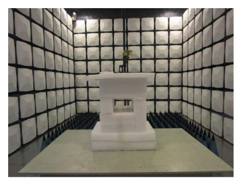
Radiated Emission View (Below 1GHz)-Battery Mode
