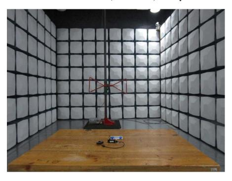
Radiated Emission View (Above 1GHz) -Battery Mode
