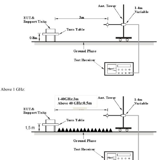
The radiated emission and out of band emission tests were performed in the 3 meters chamber test site, using the setup accordance with the ANSI C63.10-2013 The specification used was the FCC 15.209/15.205 and FCC 15.255 limits.
