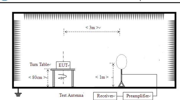
2) For radiated emissions from 30MHz to1GHz
