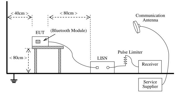
The Table-top EUT was placed upon a non-metallic table 0.8m above the horizontal metal reference ground plane. EUT was connected to LISN and LISN was connected to reference Ground Plane. EUT was 80cm from LISN. The set-up and test methods were according to ANSI C63.4:2009
