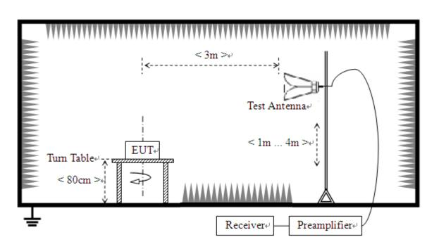
The test site semi-anechoic chamber has met the requirement of NSA tolerance 4dB according to the standards: ANSI C63.4 (2009). The EUT was set-up on insulator 80cm above the Ground Plane. The set-up and test methods were according to ANSI C63.4.
