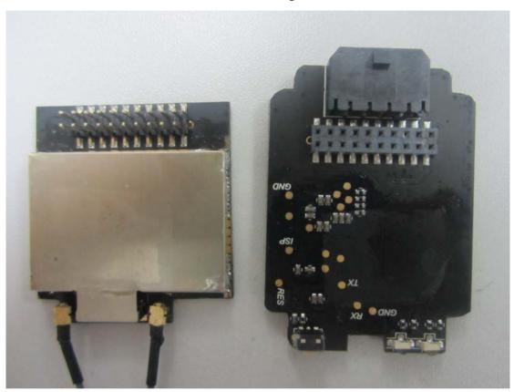
3. Mainboard front view without shielding
