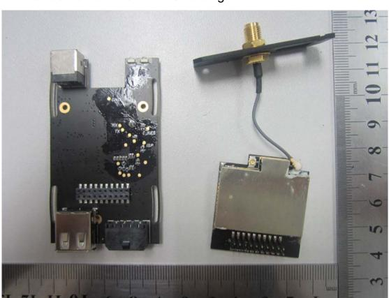
2. Mainboard front view with shielding
