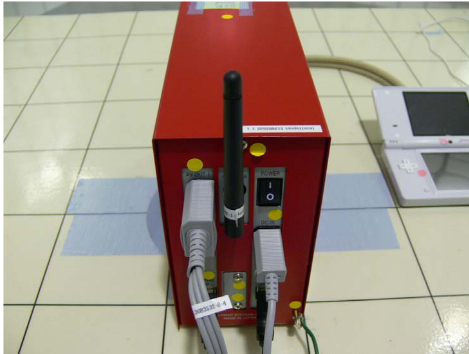
Photograph 4: Set-up for Radiated Emission, EUT Configuration Z-Axis
