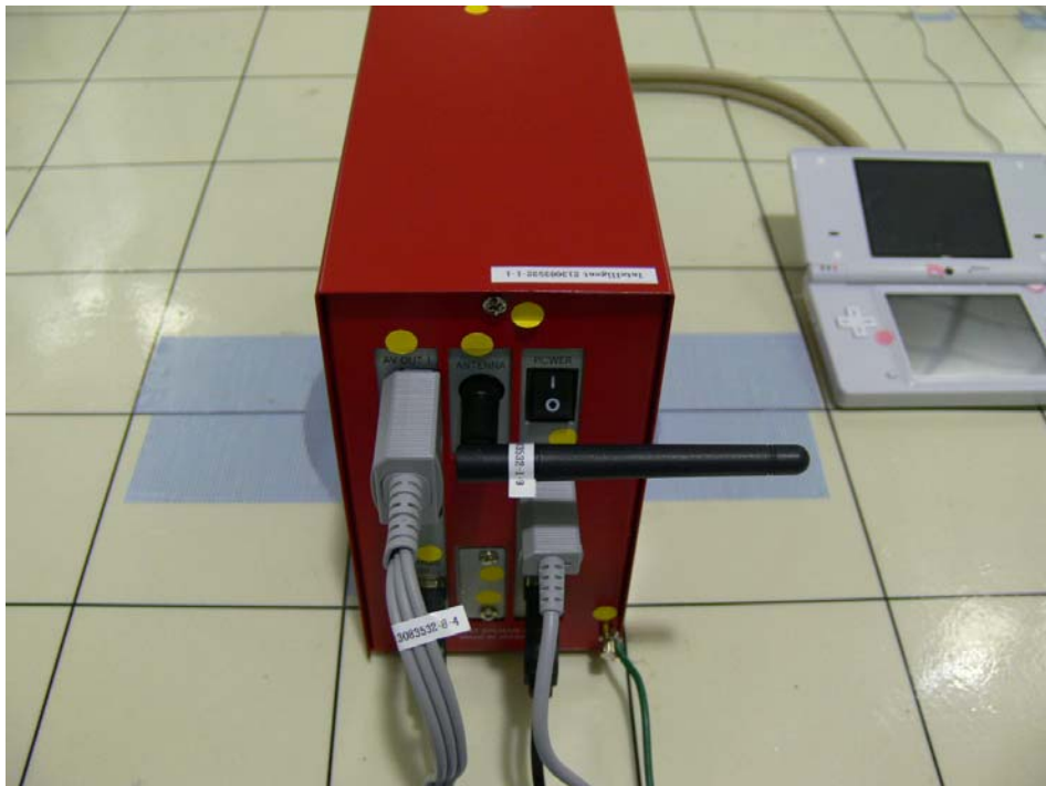
Photograph 3: Set-up for Radiated Emission, EUT Configuration Y-Axis
