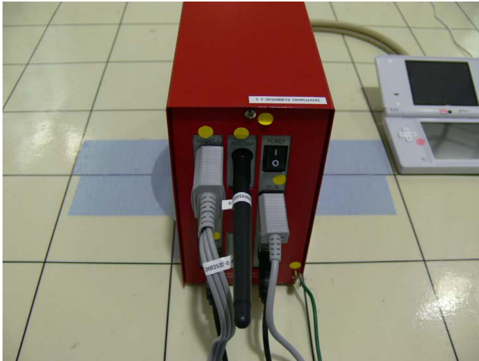
Photograph 2: Set-up for Radiated Emission, EUT Configuration X-Axis
