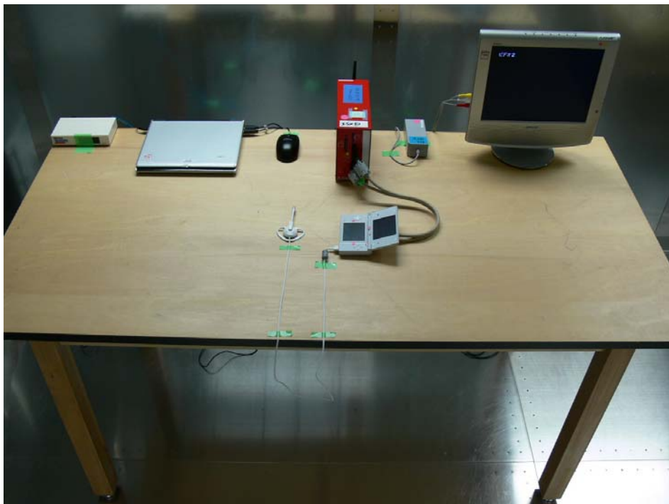
Photograph 5: Set-up for AC Mains Conducted Emission of Transmitter, Front View
