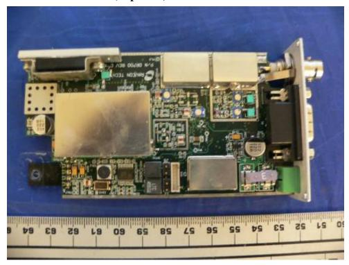
**EUT – TX Main Board shield off (Top View)**
