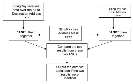
One effect of this is that an address mask of 0000 will cause the *StingRay* modem to received any data from any unit that transmits. The Destination Address will effectively be ignored if the mask is set to 0000.
