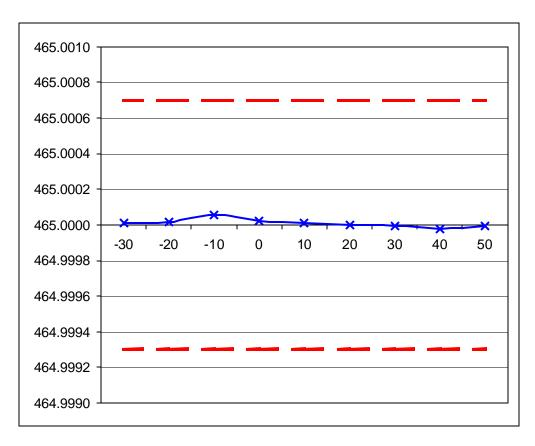
Vertical Axis = Frequency MHz Horizontal Axis = Degrees Centigrade
