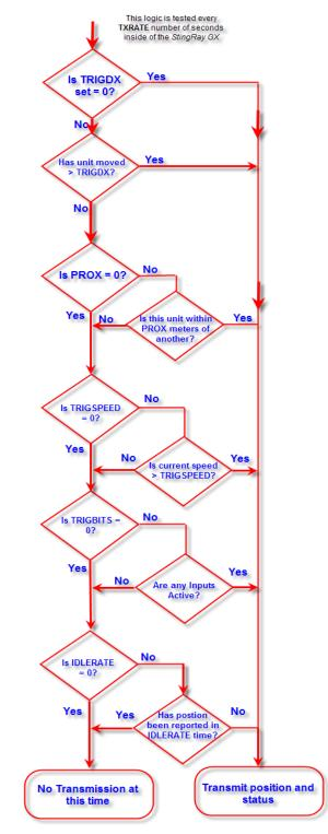
ATLAS PT Transmission Trigger Diagram
