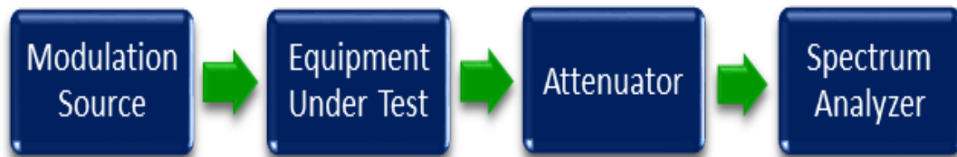
Figure 2: Modulation Characteristics Bandwidth Test Setup
