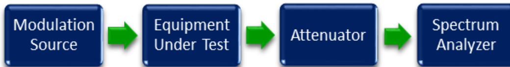
Figure 3: Occupied Bandwidth Test Setup
