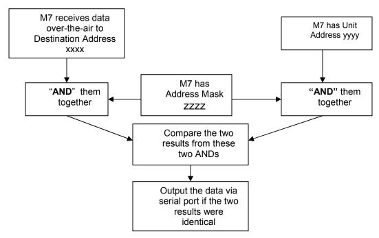
One effect of this is that an address mask of 0000 will cause the *M7* modem to received any data from any unit that transmits. The Destination Address will effectively be ignored if the mask is set to 0000.
