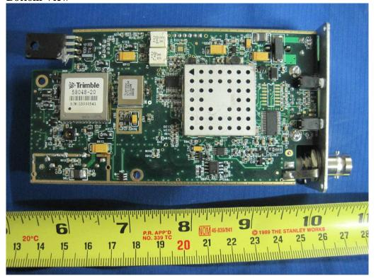
PCB Board-without RF shield
