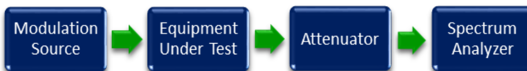
Figure 3: Occupied Bandwidth Test Setup
