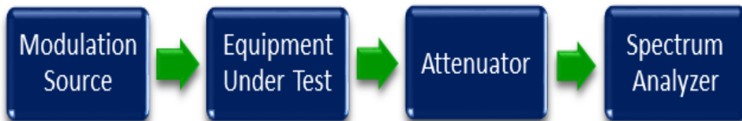
Figure 2: Modulation Characteristics Bandwidth Test Setup
