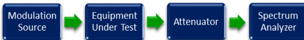
Figure 3: Occupied Bandwidth Test Setup
