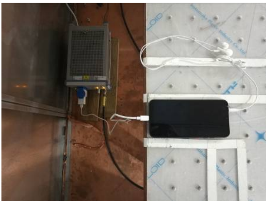
Conducted Emissions Test Setup (with charger)
