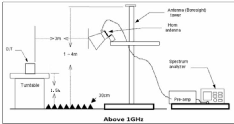
Above 18 GHz shall be extrapolated to the specified distance using an extrapolation factor of 20 dB/decade from 3m to 1m.
