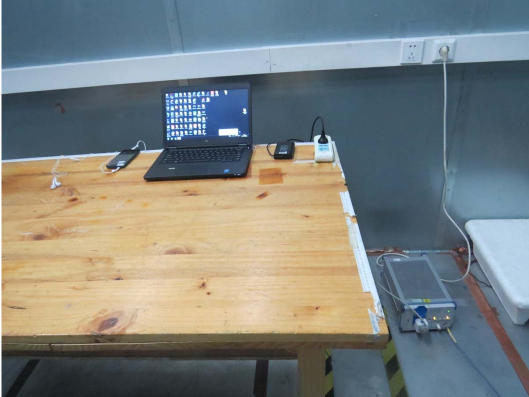
Picture 2 Conducted Emission Test Setup
