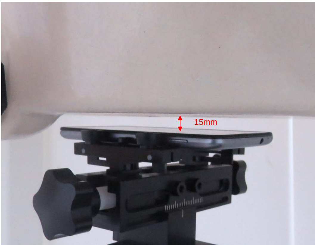
Picture 8: Front Side, the distance from handset to the bottom of the Phantom is 15mm
