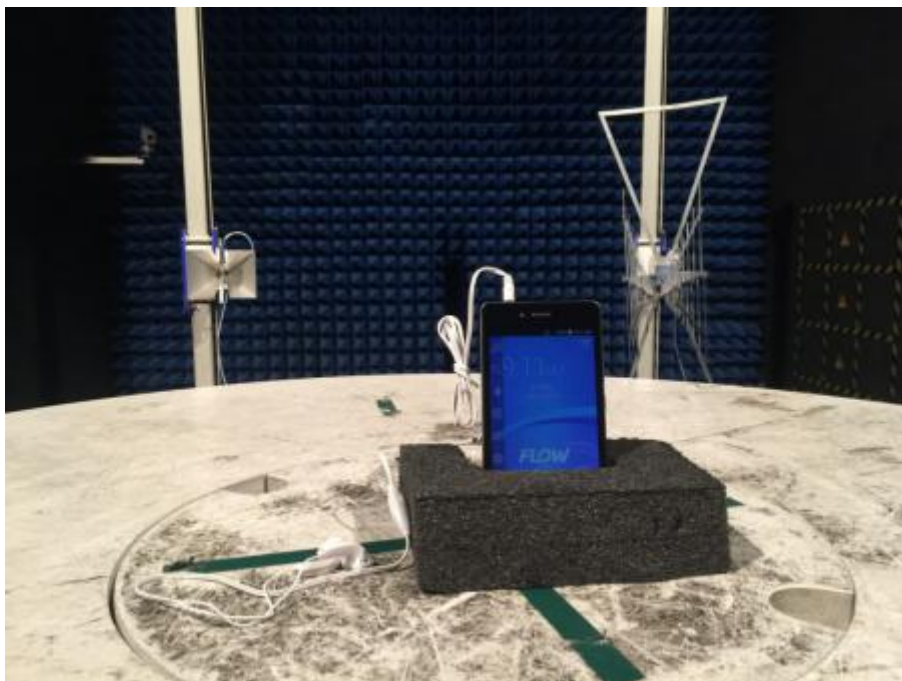
Radiated Spurious Emissions Test setup
