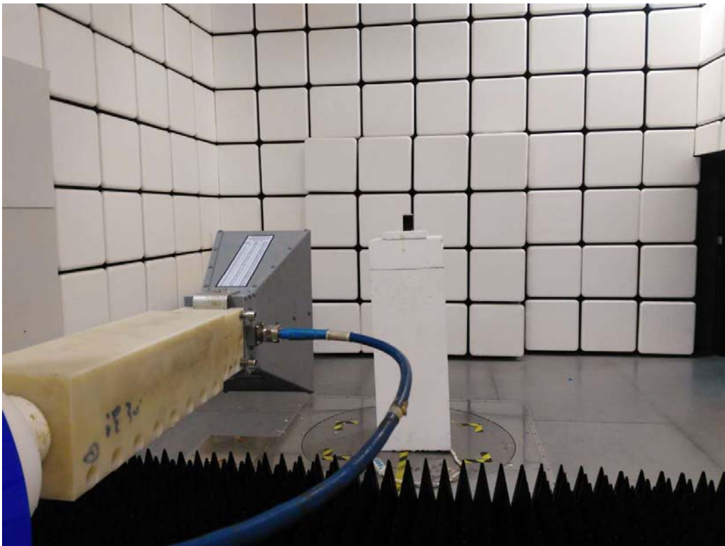
Picture 2: Radiated Spurious Emissions Test setup
