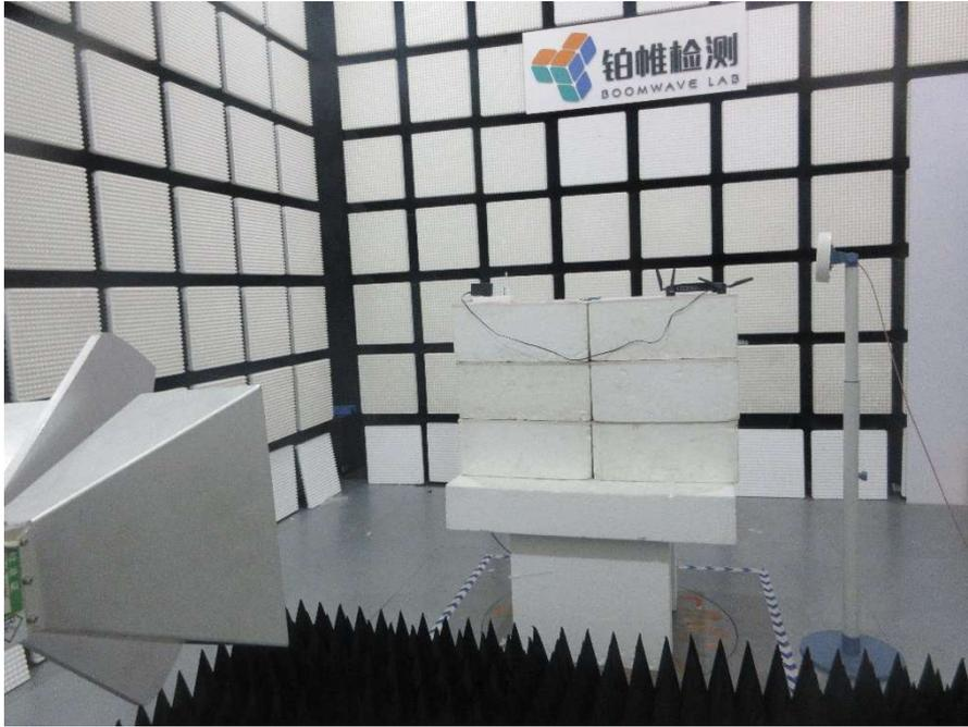
**Radiated Emission 1GHz-18GHz (Rear view) – Mode 2**
