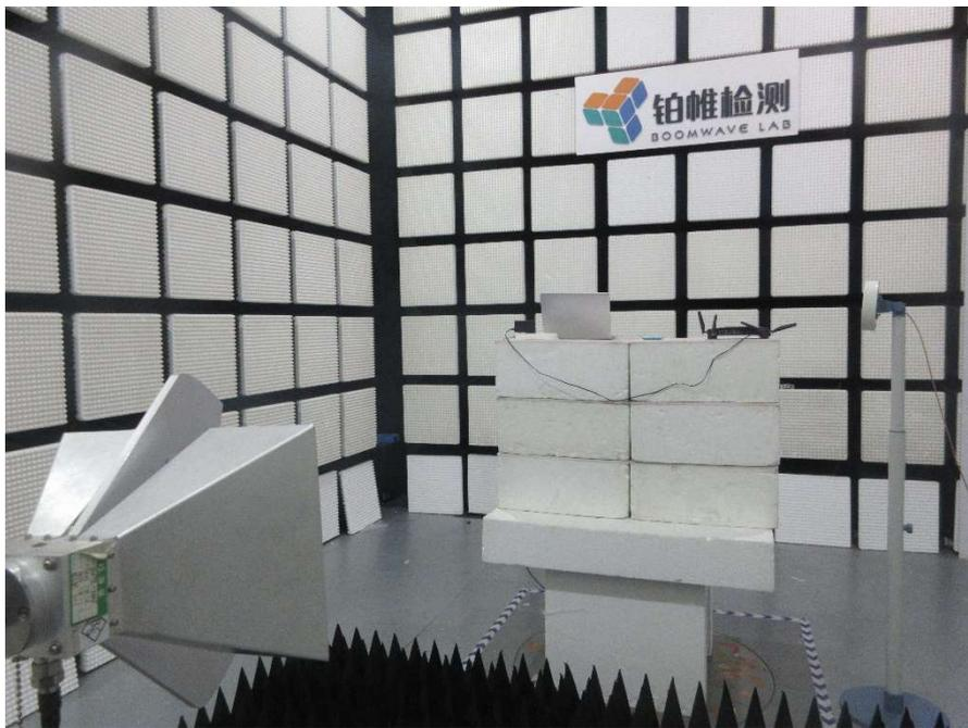
**Radiated Emission 1GHz-18GHz (Rear view) – Mode 5**
