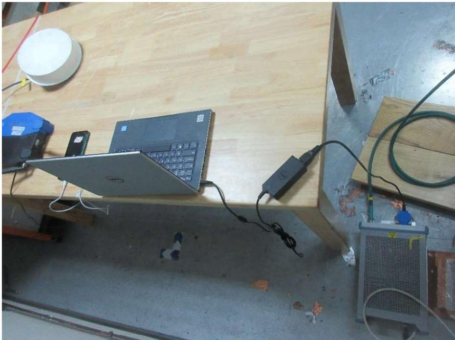
**Conducted Emission 150kHz-30MHz (Rear view) – Mode 5**
