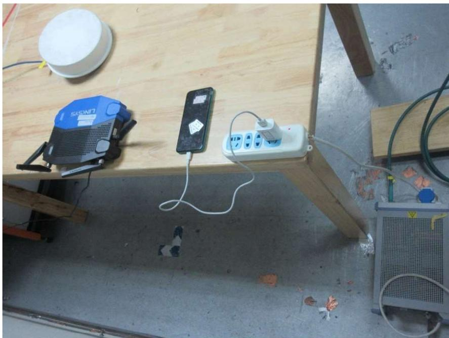
**Conducted Emission 150kHz-30MHz (Rear view) – Mode 2**
