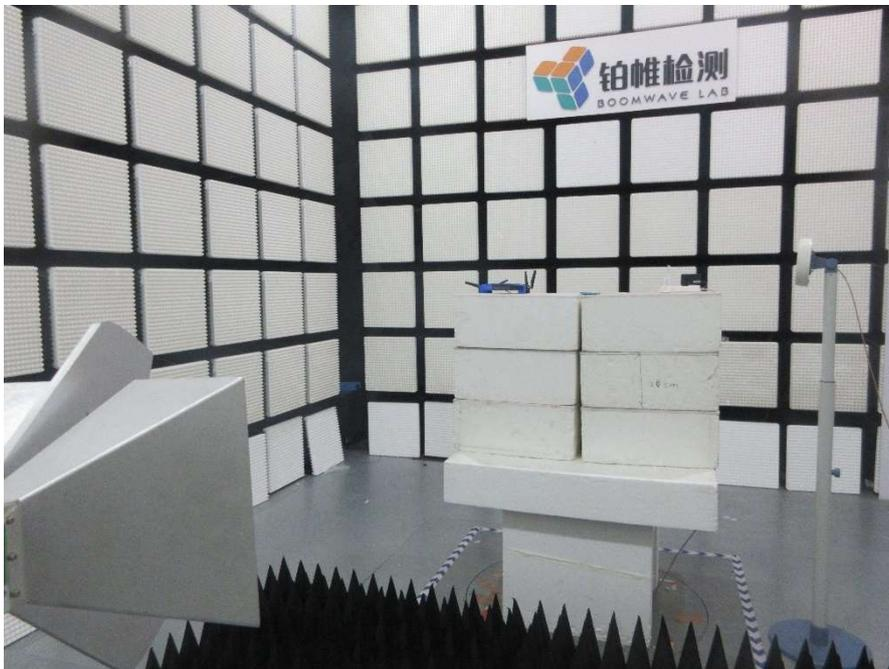
**Radiated Emission 1GHz-18GHz (Front view) – Mode 2**
