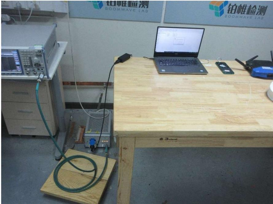
**Conducted Emission 150kHz-30MHz (Front view) – Mode 5**
