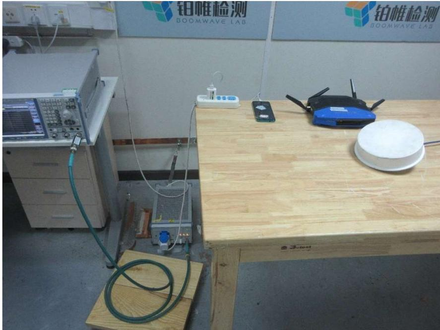
**Conducted Emission 150kHz-30MHz (Front view) – Mode 2**
