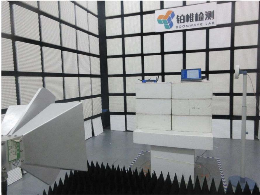
**Radiated Emission 1GHz-18GHz (Front view) – Mode 5**
