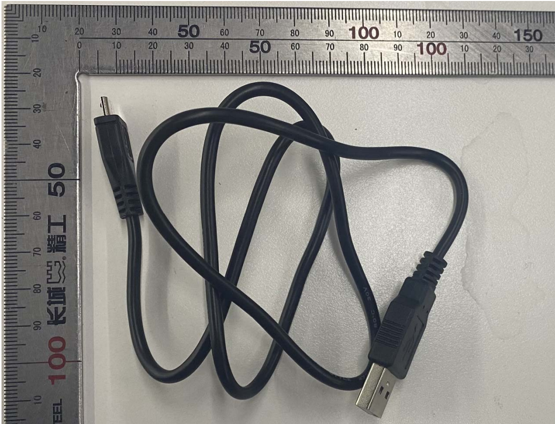
USB Cable(V815W-USBMicro USB_L=0.7m black_low level made by Dongguan Guojun Plastic Electronic Co.,Ltd)
